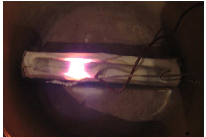
Figure 8. The local overheating that leads to reactor's failure.
