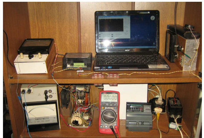
Figure 3. Equipment for heater powering and diagnostics. Left to right on the upper shelf: thermocouple signal amplifier with power regulator, the data logger, the computer for recording temperature and rate of Geiger counter, device for measuring the rate of Geiger counting. Left to right on the lower shelf: amperemeter, reactor's power source, voltmeter, watt-hour meter, power line switch.
