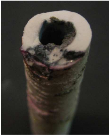
Figure 9. Fragment of the reactor, destroyed due to local overheating.
