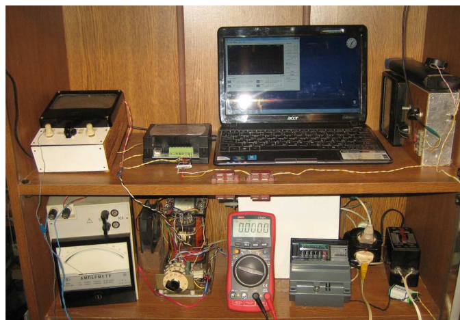
Figure 3. Equipment for heater powering and diagnostics. Left to right on the upper shelf: thermocouple signal amplifier with power regulator, the data logger, the computer for recording temperature and rate of Geiger counter, device for measuring the rate of Geiger counting. Left to right on the lower shelf: amperemeter, reactor's power source, voltmeter, watt-hour meter, power line switch.
