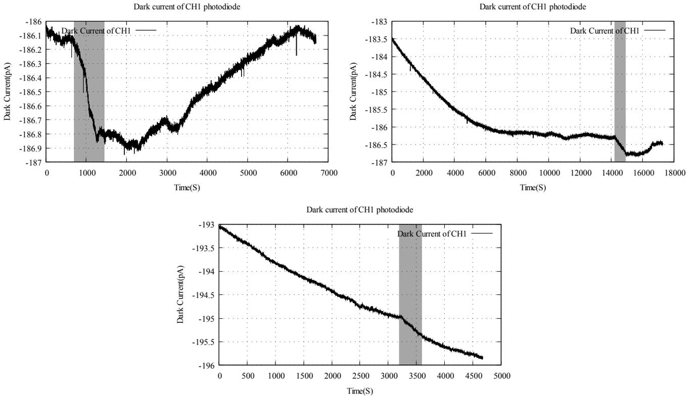
Figure 11. The local tests with blue LED generator. Distance between sensor and generator is 10 cm. Grey area means the impact time.
