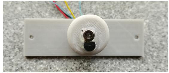
Figure 24. The configuration of temperature sensor inside.
