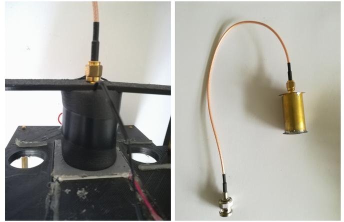
Figure 6. Sensor with thermostat (left); Sensor cell (right).
