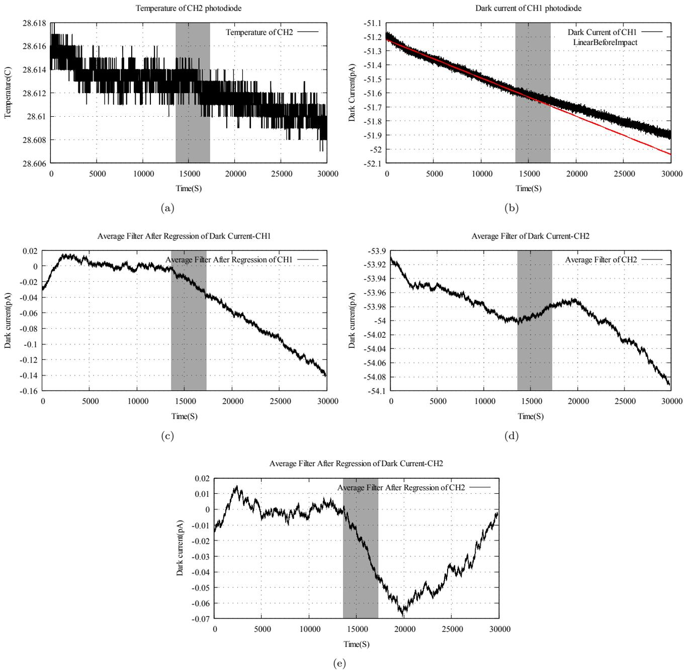
Figure 16. Exp20170918: Non-local test with spinning Poynting vector generator, distance between sensor and generator is 5km, non-local link is the photo of CH2. Grey area means the impact time. Polarization: right-handed. (a) temperature of both channels; (b) data of CH1; (c) filtered data with 120 points after linear regression of CH1; (d) filtered data with 120 points of CH2; (e) filtered data with 120 points after linear regression of CH2.
