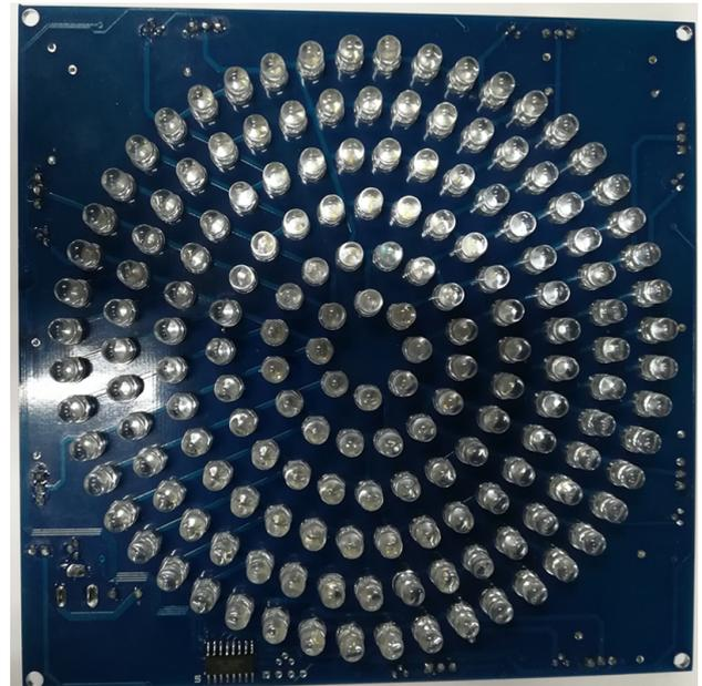
Figure 3. The LED generator used in experiments.
