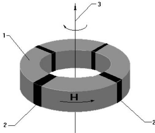
Figure 1. Basic structure of the rotator in the spin field generator. 1 - Ferrite ring 20x12x6 mm, 2 - ferrite-barium magnets, 3 - the rotation axis.
