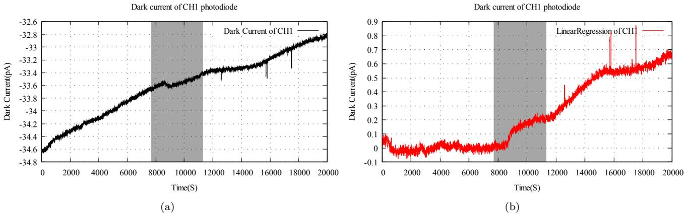
Figure 12. Non-local test with blue LED generator, distance between sensor and generator is 3km, non-local link is the photo of photodiode in the sensor. Grey area means the impact time. (a) is original data; (b) is linear regression of data.
