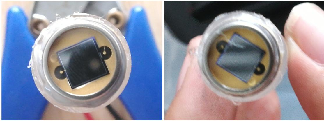
Figure 17. Two photos of photodiodes in the two channels of the sensor.
