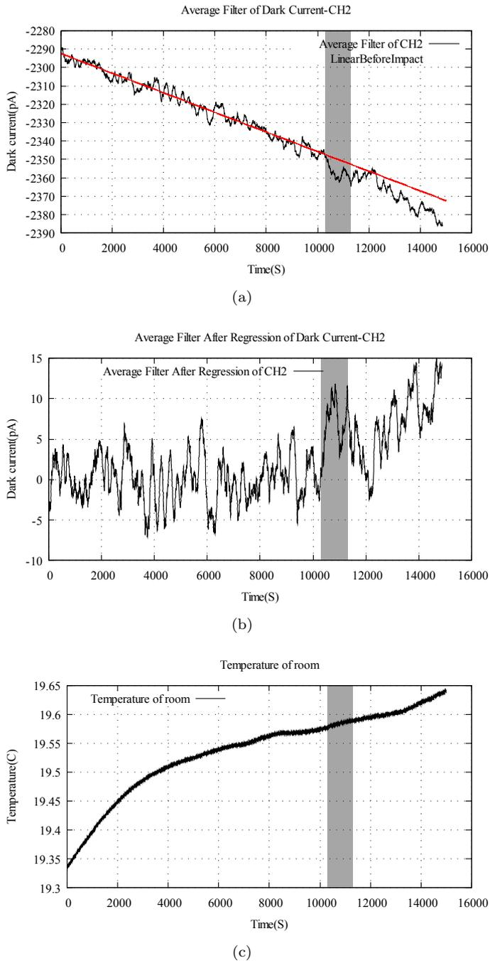
Figure 23. Exp20171209: Non-local test on the avalanche photodiode with spinning Poynting vector generator, distance between sensor and generator is 5km, non-local link is the photo of avalanche photodiode. Grey area means the impact time. Polarization:right-handed. (a) filtered data with 120 points and linear calculation for the part before impact; (b) filtered data with 120 points after linear regression; (c) temperature of room.
