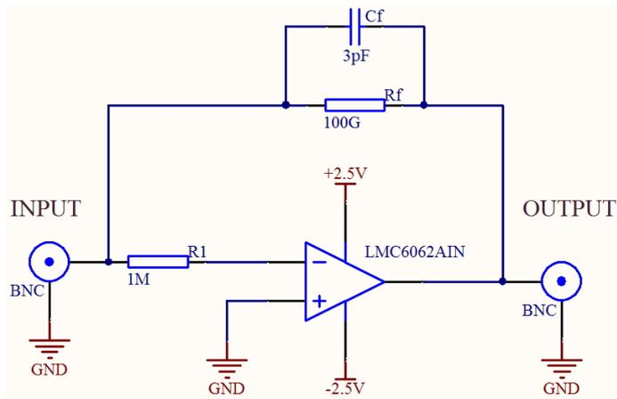
Figure 7. The core schematic diagram of the ultra weak current meter.
